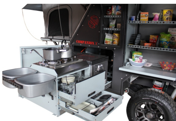
Perfectly laid-out kitchen with easy to reach fridge, instant hot water wash-up facility and a large grocery cupboard with space for a microwave.
